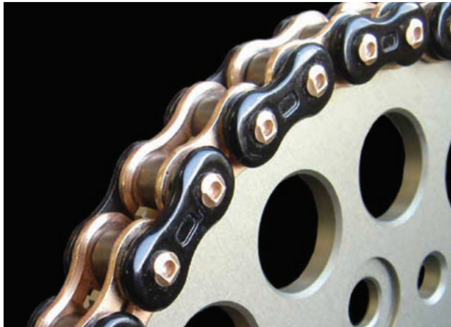
O-ring chains seal lubricant inside the pin bushings, and these seals help keep out impurities. This extends chain life, but doesn't eliminate the need for lubing and cleaning.
