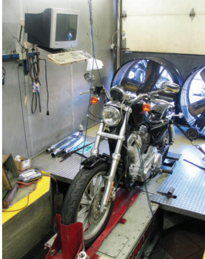
A dynamometer measures both horsepower and torque. The data are recorded in 500 rpm increments, or sometimes at 250 rpm increments, and the horsepower line is calculated.
