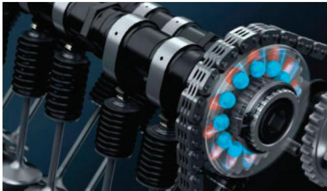
Suzuki's SR-VVT system was designed to be legal in MotoGP racing. Available on its 2019 GSX-R1000 sportbikes, the mechanical system nonetheless creates smooth advance transitions—ideal for racing at the limit.
