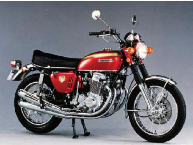
The 1969 Honda CB750 Four was a game-changer. Cylinders were tilted forward, lowering center of gravity and increasing space.
