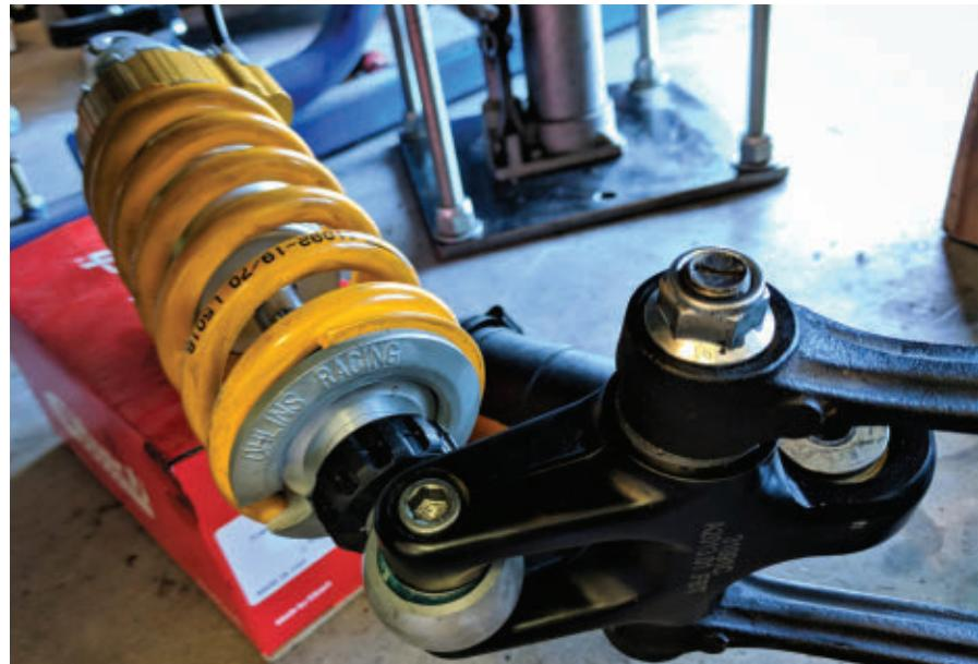
**Samantha installed an Öhlins shock, which didn't fix harshness and bucking issues.**
