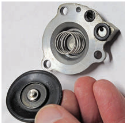
The accelerator pump shoots an extra burst of fuel when needed, helping to avoid a low-speed lean sputter.
