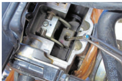
Jet needles and e-clips are accessed and removed easily with pliers from the top of the carburetor.
