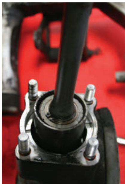
Regular lubrication and maintenance of the pinion/ring gear could end up saving the bike owner replacement costs of $1,000-$1,500 for a new gearbox.
