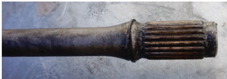
This male shaft spline shows the result of not having enough grease, which is a drive shaft's worst enemy. Here, moisture has caused rust and excessive wear.
