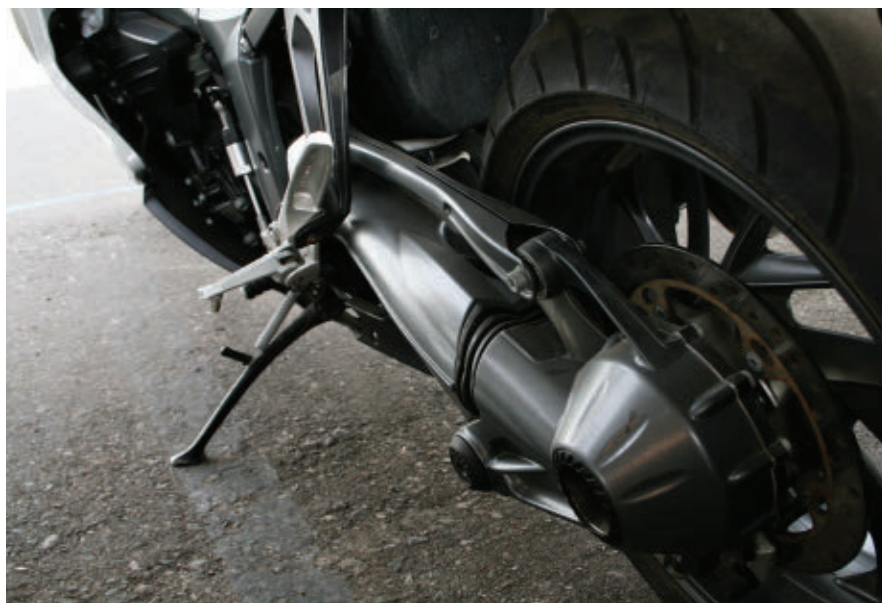
Shafts are most often found on long-range, touring-type motorcycles and have several advantages, such as durability and low maintenance.
