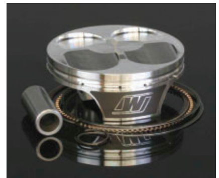
Illustrating the latest friction reduction strategies, this aluminum piston from Wiseco uses lightweight forged construction, a short wrist pin, anti-friction coatings on the skirts and very narrow low-tension rings.
