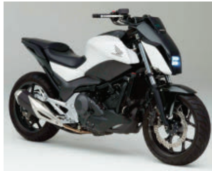
Honda's self-balancing motorcycle uses what the company calls "Riding Assist" system, using technology from its robotics research program.
