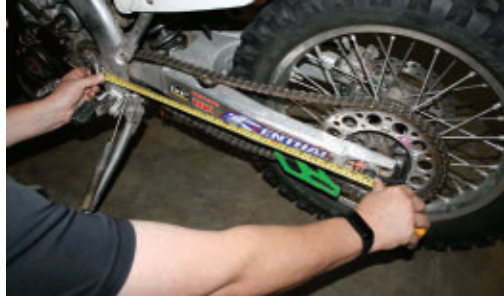
To align the rear axle, measure from the center of the swingarm pivot point to the center of the axle on both sides. The length should be the same.
