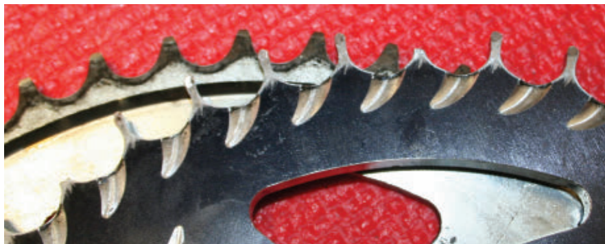
Check sprockets for broken teeth or abnormal wear. All teeth should have a uniform, equidimensional, tent-like shape.
